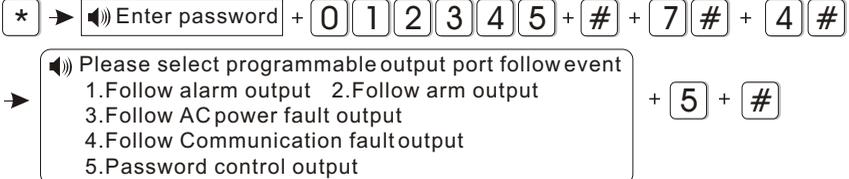
Hint: when setting as password control output, press key5 for 3 seconds, then enter the user password, the programme output port will be open or closed. Voice phone or SMS also can open or close the outport.
