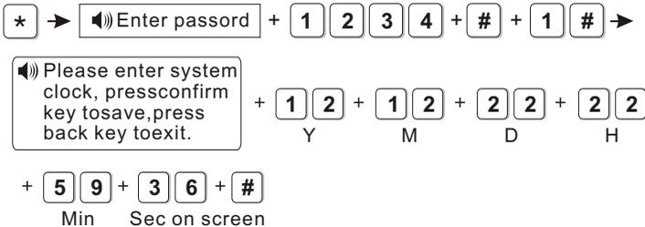
According to flash of Y.M.D.H.Min.Sec on screen, enter 12.12.22.22.59.36 by turn, also can press [UP] [DOWN] key to move cursor.
