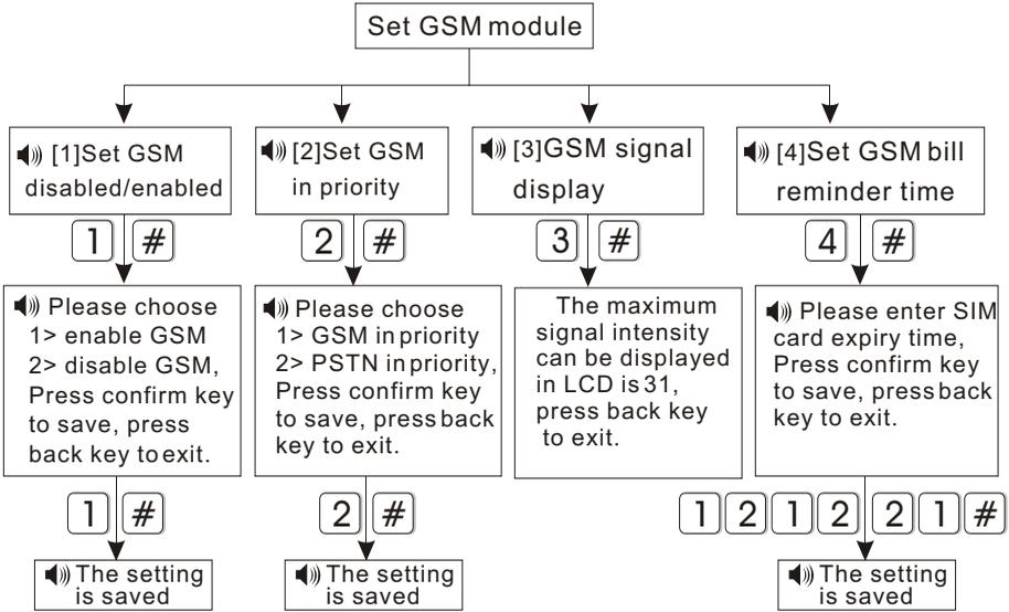
Hint: The alarm control panel will send SMS to cellphone as preset and remind you to recharge as you set GSM bill reminder time before or after ten days.
